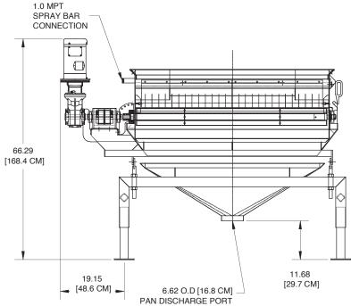
2. ROLLER BED CAN BE TILTED +/- 4 DEGREES WITH SCREW ADJUST SUPPORTS AT INLET END
